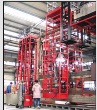
AGWII-LNG with engine welder trailer
