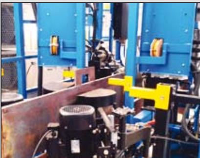
Buff Equipment for joint cleaning prior welding
