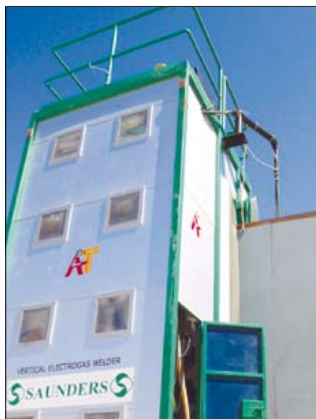
EGWII rides on shell for conventional bottom up tank welding
