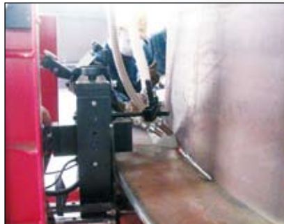
All Time girth welder with elevated weld head assembly to weld multiple stiffeners on the same vertical structure
