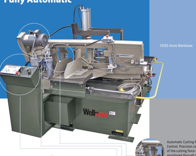
unattended automatic operation with the versatility of a swivel head for miter cuts. Operation requires very little training and is quick to set up in either automatic or manual sawing modes.
